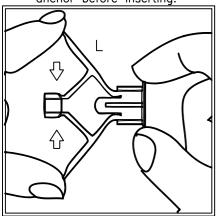
Insert the chuck into the hole of the base material.
