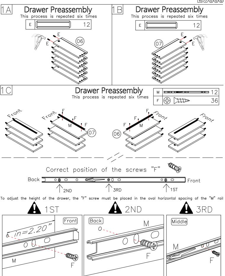
Use the indent as a guide for installing the rails
